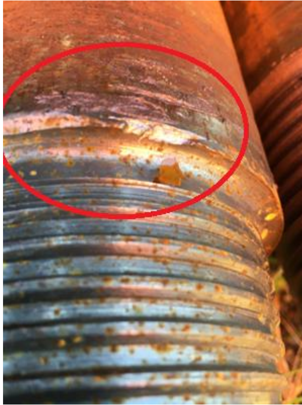
Seal face damage, caused by possible impact or over bend
