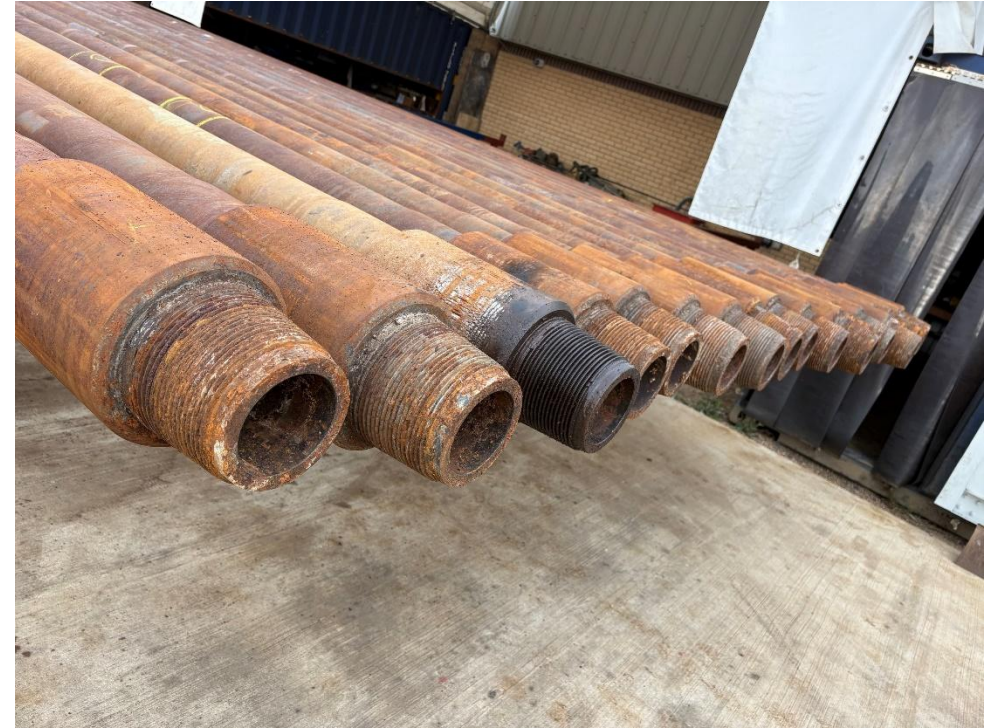
Impact damage and corroded threads
