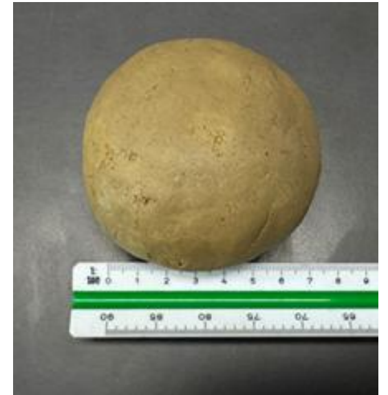
Pugging ball from native backfill after 10 months
