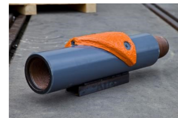
Figure 14: Weeper sub ready for use.
