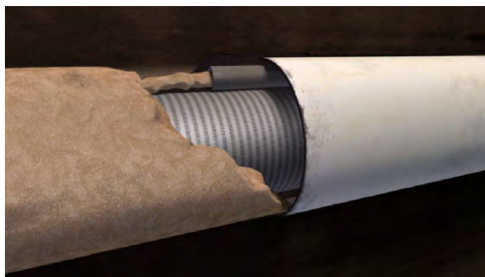
Fig. 9: Gravel packing the screen and borehole during retraction of the casing pipe
