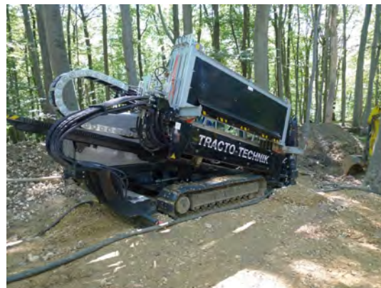
Fig. 13: Grunddrill 18ACS of WMZ-Company on top of the gorge
