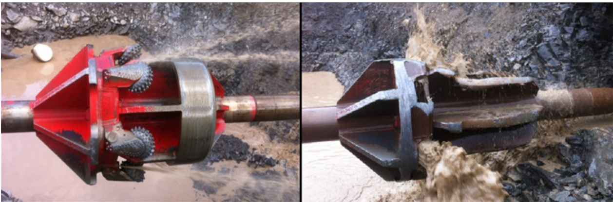
Two pictures of the same tool after 4 resp 79 hrs in the hole
