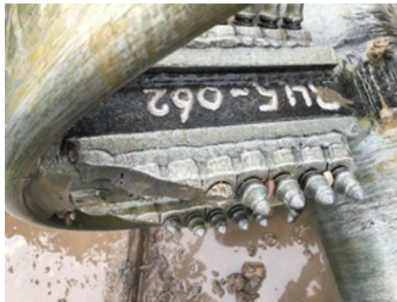
Wear on fly cutter. Note all teeth on outer ring are gone
