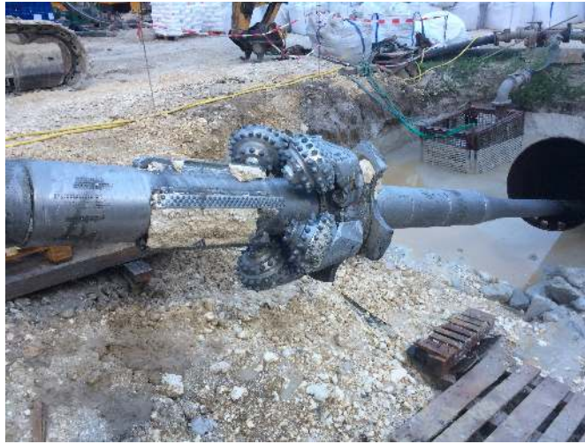
Picture 04: Hope Opener after reaming HDD1
