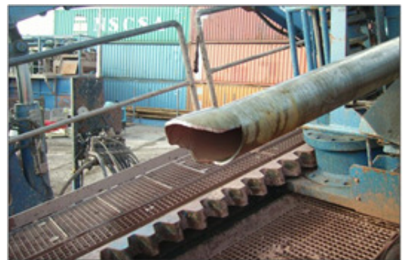
Broken drill pipe
