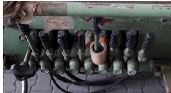
Figure 2: Control unit of an old drilling rig
